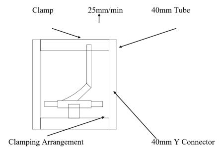
Prepare an assembly as above and using a suitable clamping arrangement secure the 40mm protective tube section to one of the tensometer jaws. Place the branch tube in the other jaw and perform a destructive test at a rate of extension of 25mm/minute.
